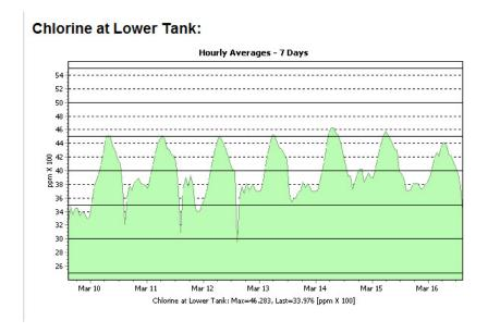
The variations upward are when freshly chlorinated water arrives into the lower tank during the night, which then somewhat dissipates until the process repeats the next night. All water in the new tank at the Overlook is pumped from the lower tank, and so the chlorine residual levels are relatively even throughout the entire system.
